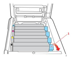
**6.** Lift the right-hand end of the cartridge and then draw the cartridge to the right to release the left-hand end as shown, and withdraw the toner cartridge out of the MFP.
